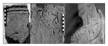
Figure 7. Bricks from the 120-250 CE gates at Halin. Fingermarks (left), letter a (centre), number 90 (right).
